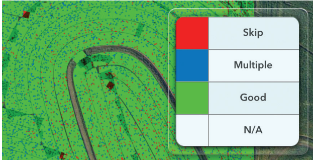
Field planted in 2014 with finger meter. Average singulation was 96.2%, skips were 1.5% and multiples were 2.3%.
